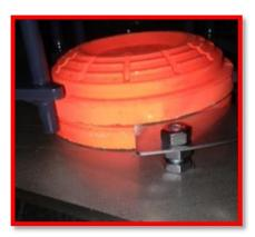
(f) When loading the clays be sure there are no tight spots in the carousel. Occasionally machines can suffer slight damage to the carousel.
