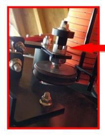
There is spring tensioner on the bogie wheel that can be adjusted to help transfer clays over the holes in the top plate. This will come set from factory but may need adjustments over time.
