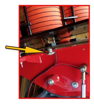
**Step 16** – The pull cord or optional wireless release can now be connected to the machine. The manual pull cord or wireless release gets connected to the yellow-ended cord plug.
