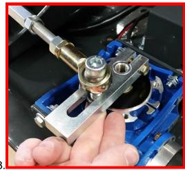
**Step 15** – You can adjust the distance that the clay is thrown by extending the spring. This is achieved by winding tension on or off the main spring using a ¾" wrench or the optional ¾" extended socked which can be attached to an impact drive. This should be done with the machine in the disarmed/safe condition for small adjustments. **AFTER ADJUSTING THE MAIN SPRING FOR THE CORRECT THROWING DISTANCE, THE NUTS ON THE SPRING STUD MUST BE TIGHTENED SECURELY AGAINST EACH OTHER.**
