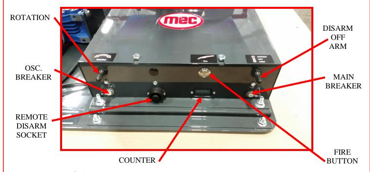
**Rotation Toggle Switch** – Pushing the switch downward will turn the oscillation motor on. Note that the oscillation motor will randomly start/stop when the machine is in operation. This prevents shooters from being able to predict the direction of the next target. Pushing the toggle switch upward allows you to nudge the oscillation motor which pivots the machine from one side to the other enabling you to check the angle of the clays flight.
